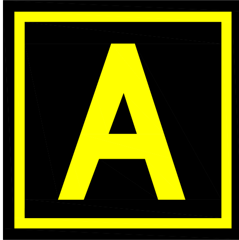
(a) Taxiway Location Sign
